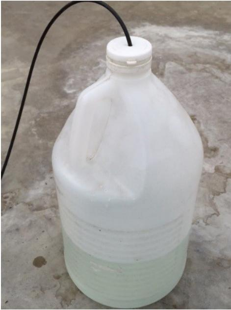
Figure 8. Gallon jug used to collect irrigation leachate.
