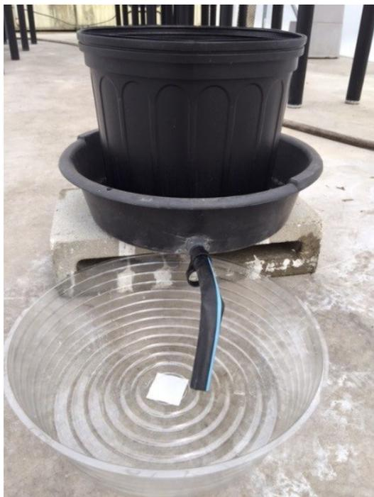
Figure 5. Using an oil pan drain to catch leachate.
