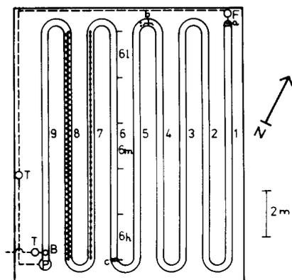
Fig. 1. Schematic diagram of a deep, circulating, water-culture system. 1—9 = number of channel sections (rows); a, b, c = aeration points; 6h, 6m, 6l = sections of Row 6 with high, medium and low  $O_2$  concentrations, respectively; B = float; F = flowmeter; P = pump; T = tap; broken line = water tube; dotted line = aeration by an air tube with in-line drippers; heavily dotted line = aeration by porous air tube.
