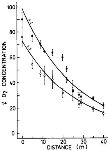
Fig. 2. Change of  $[O_2]$  with distance from aeration point in a deep circulating hydroponic system. Rates of water flow were  $4.5 \text{ l min}^{-1}$  (○) and  $6.2 \text{ l min}^{-1}$  (●). Vertical lines are standard deviations.
